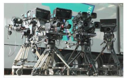
TopVision 3D Cameras on Mirror Rigs and on Side-by-Side Rigs
